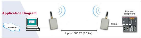
This is the simplest and easiest way of setting up the RF wireless unit. Simply configure the units with the included configuration software and they are ready for use.
