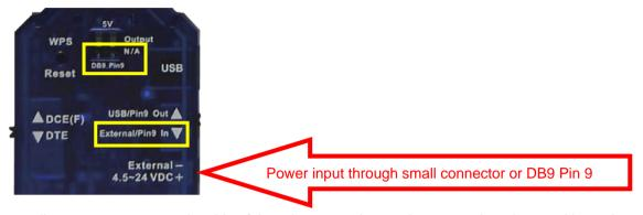
The small power connector on the side of the adapter can be used to power the adapter with a voltage raging from 4.5 to 24VDC.
