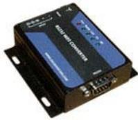
The Bit Commander US2000A/B is a light-industrial grade serial RS232 / RS485 to Ethernet converter which can be used to connect any standard RS232 or RS485 serial device to a computer over a standard Ethernet network. It has a strong aluminum housing with screw mounting holes for easy installation which makes it ideal for most factory environments and other commercial facilities.
