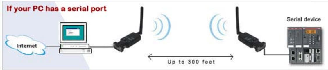
Direct cable replacement. One Master adapter communicates with one Slave adapter to create a wireless link between a computer and a serial device. Only one Slave can be connected to one Master. Often used if PC has no built-in Bluetooth.
