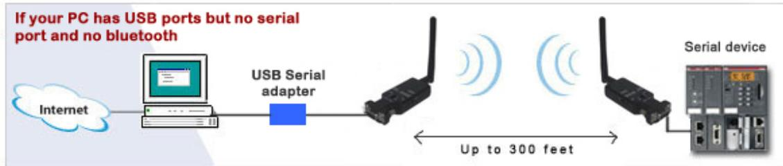
Direct cable replacement option 2. If your computer does not have a serial port you can connect the serial Bluetooth adapter to your computer by using a USB to serial adapter.
