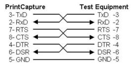
If your test equipment is configured as DCE you will need a cable to connect DTE to DCE, or what is referred to as a "straight-through" cable, as shown below for 9-pin serial connectors. Use a Belkin F2N209 or equivalent for this cable.
