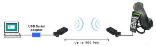
You will need two serial Bluetooth adapters (part UCBT232B). The local (master) serial Bluetooth adapter is connected to your computer by using a USB to serial adapter (part XS8801). The remote (slave) serial Bluetooth adapter is connected to the hand control via a RJ11 to DB9 female cable. The hand control is then connected to the telescope mount.
