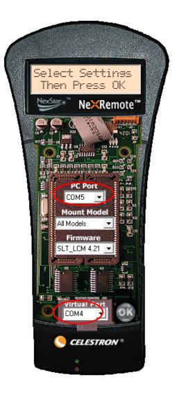
In NexRemote also select the mount model, firmware and virtual port; then click the OK button. In Windows Device Manager you should now be able to see the virtual COM port created by NexRemote. This is also the COM port which will be used by ASCOM.
