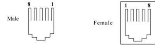
RJ-45 connection diagram
